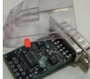
**Figure 6. Internal clamshell and PCBA.**
