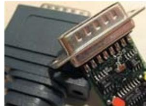
**Figure 7. Overmold PCBA solution.**
